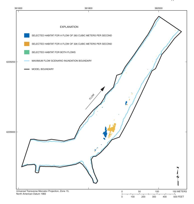
Figure 3-80. Selected habitat area distribution for habitat categories 16, 17 combined (channel catfish) at flows of 283 and 326 cubic meters per second at Marais des Cygnes River site MDC1.
